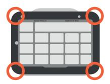
Push all four corners firmly to make sure the keyguard is secured.
