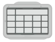
Place the perspex keyguard on the front of the device.
