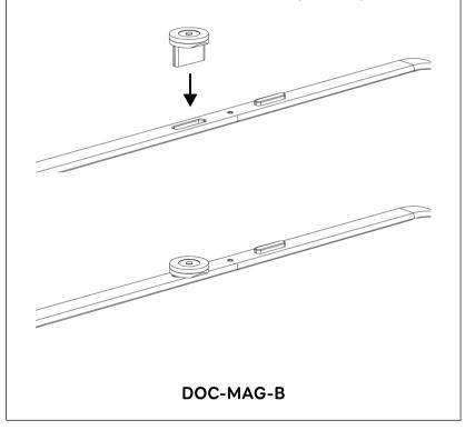
2. The cable will connect magnetically to connector.
