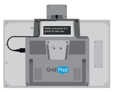
5. (Optional) Use the cable clips to fix the USB cable to the back of your Grid Pad, to prevent it getting caught when moving the device. We have provided 2 cable clips with sticky adhesive backs.
